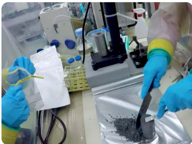
State-of-the-art contamination control was used for microbiological sampling from sediment cores during International Ocean Discovery Program Expedition 370. In order to avoid the intrusion of drilling fluid into the inner part of the “mbio” sample, the outer part was carefully removed with sterile tools inside an anaerobic chamber. From Heuer et al. (2019), https://doi.org/10.5670/oceanog.2019.147
